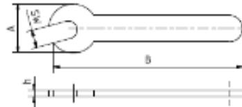
Open-end Wrench for Nuts with hexagon and wrench size
